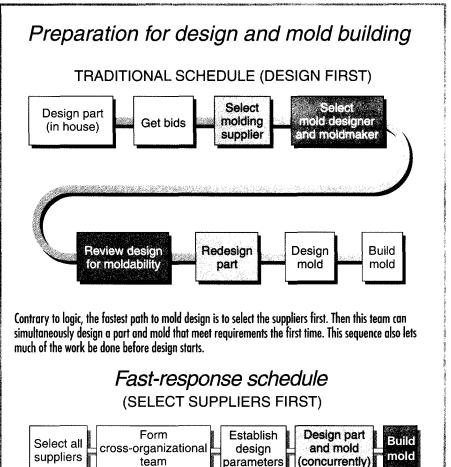
cut steel. First, the productdevelopment unit is involved. Then comes mold design which, even if done within the company, is usually performed by a separate department. Next comes the moldmaker, followed by texturing in still another organization. Finally, the molding house shoots the initial parts.
