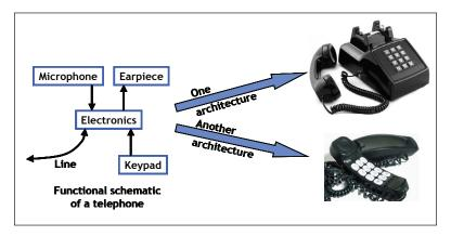
*Figure 3. Two different architectures for a corded telephone (Source: Copyright ©2007 by John Wiley & Sons; used with permission)*
