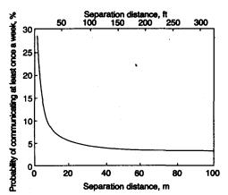
**Fig. 6** Effect of separation distance on communication between team members. Communication is much more likely to occur if team members are located within about 10 m (30 ft) of one another. Source: Ref 7
